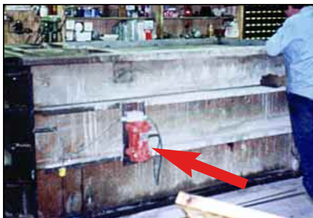
Model US-1600 permanently mounted on 5500 lb. mold.
