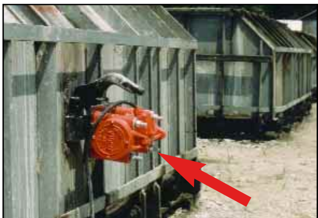
Portable US-900 on UW-2 wedge bracket for multiple septic tank forms.
