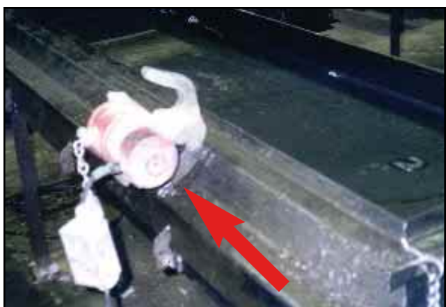
Model US-450 on wedge-bracket for vibrating lid on burial vault form.
